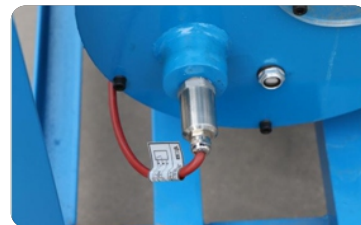
Hose leak detector
